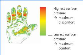
Measurement of SQ.line KERRISON bone punch's surface pressure distribution with a pressure measuring foil.
