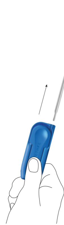
Step 2 - Press lever and remove shaft
